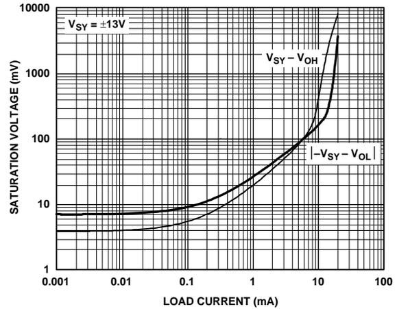
Figure 22. Output Saturation Voltage vs. Load Current
