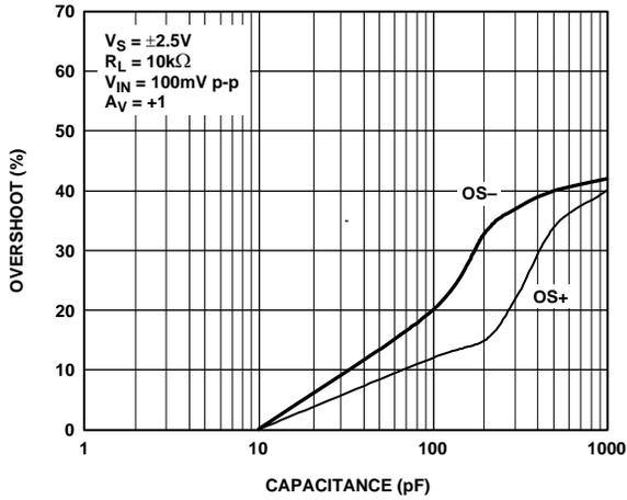
Figure 37. Small Signal Overshoot vs. Load Capacitance
