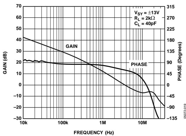
Figure 24. Open-Loop Gain and Phase Margin vs. Frequency
