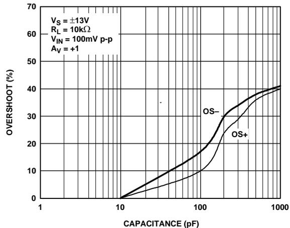
Figure 36. Small Signal Overshoot vs. Load Capacitance
