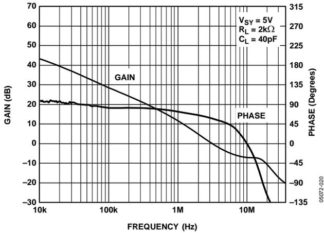
Figure 25. Open-Loop Gain and Phase Margin vs. Frequency
