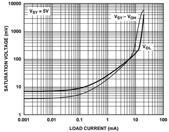
Figure 23. Output Saturation Voltage vs. Load Current
