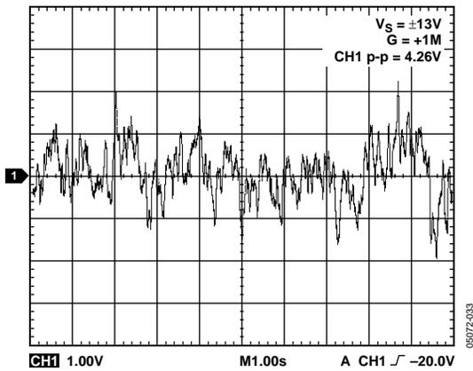
Figure 38. 0.1 Hz to 10 Hz Noise
