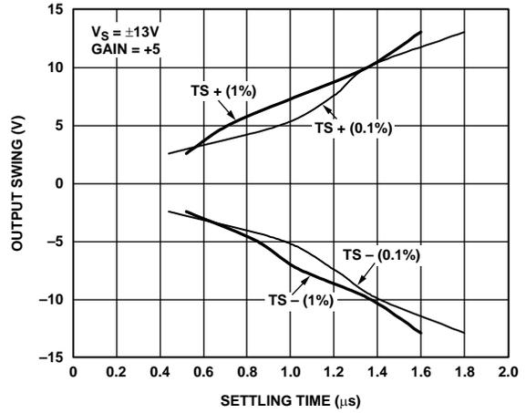
Figure 35. Output Swing and Error vs. Settling Time
