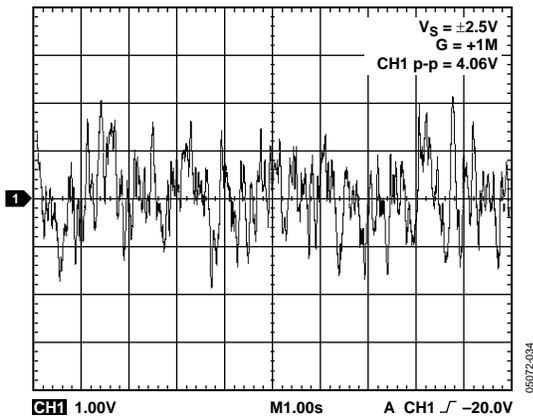
Figure 39. 0.1 Hz to 10 Hz Noise
