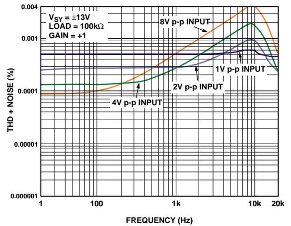
Figure 42. Total Harmonic Distortion + Noise vs. Frequency
